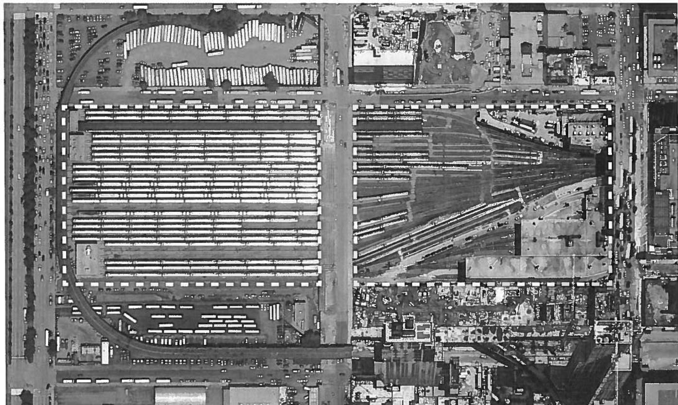
The platform and buildings above the Eastern Yard are supported by a total of 300 caissons, ranging from four to five feet in diameter and 20 to 80 feet in depth, which will be drilled deep into the bedrock in strategic locations between existing railroad tracks. The platform on the Eastern Yard utilizes 25,000 tons of steel, 14,000 cubic yards of concrete and weighs more than 35,000 tons.
